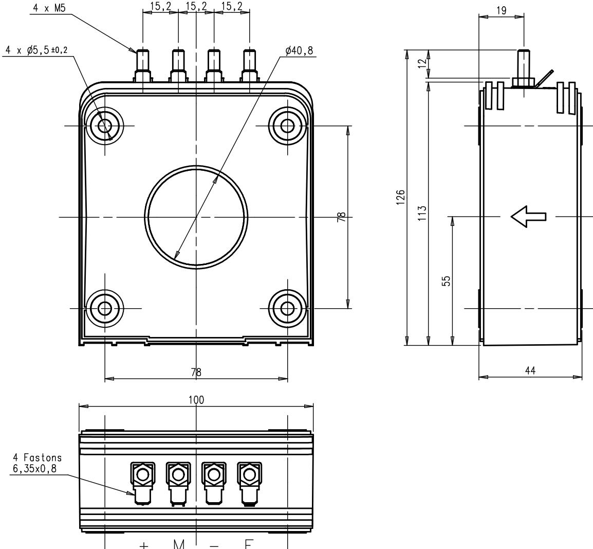
**Maximum M5 tightening torque : 2 N.m**
